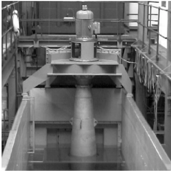
Figure 8 Turbine set-up for testing at TU Munich of WD-Kaplan turbine scale 1:3.5
