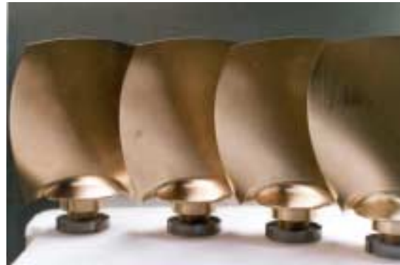
Figure 6 The runner blades of the WD- Kaplan turbine scale 1:3.5
